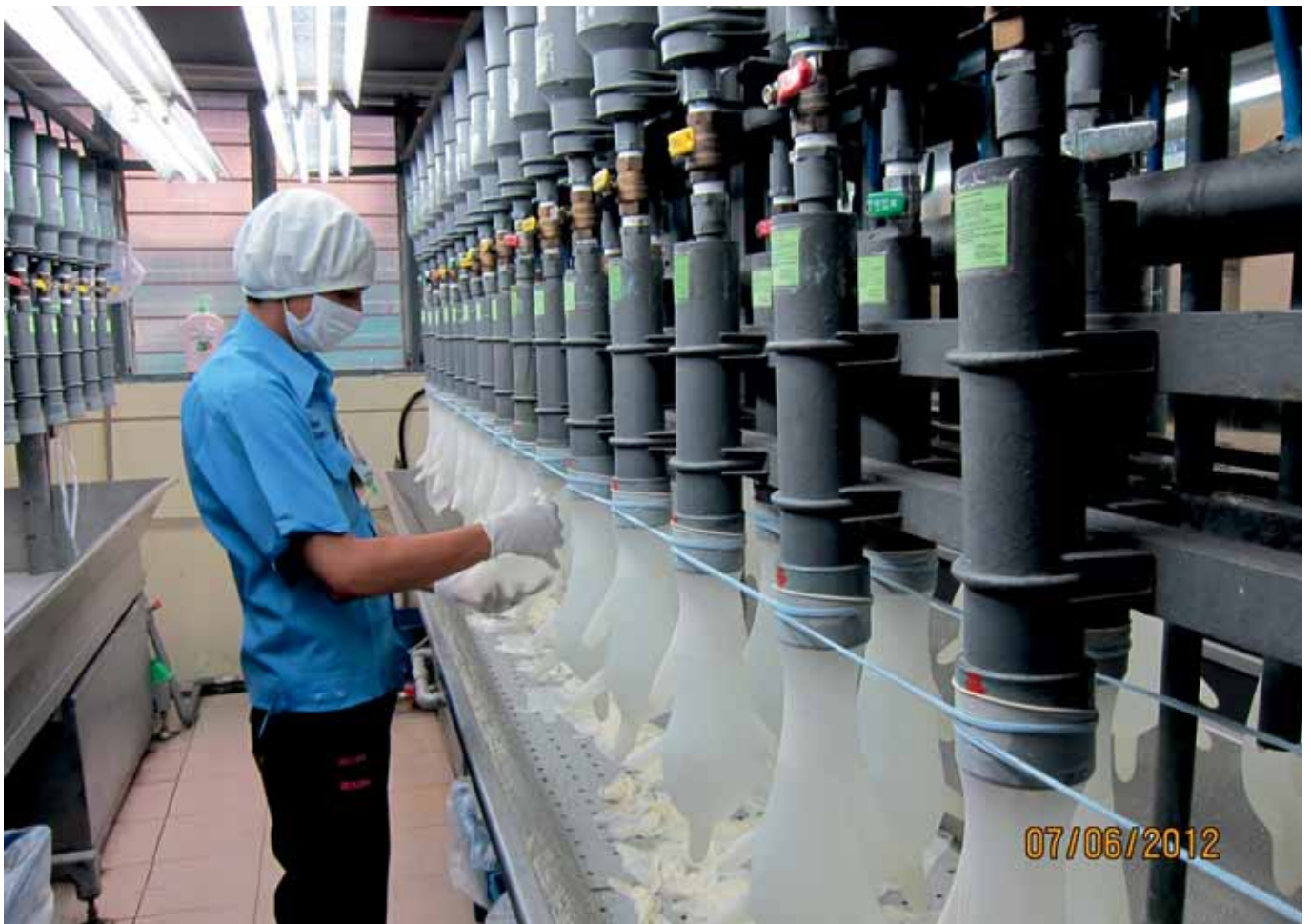
Top Glove pinhole test
